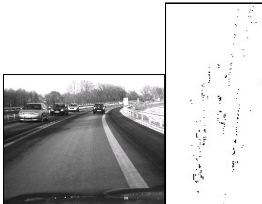
Fig. 9: Left image and the satellite view of the 3D points
