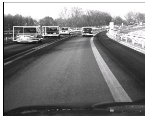
Fig. 11: Perspective view of object cuboids painted over the image
