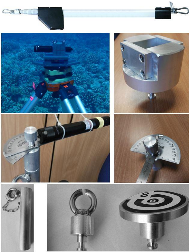
Fig. 1. Special low-cost equipment as developed for underwater surveying; from top to bottom: graduated bar for distance measurements, laser pointer on a tripod (left) and staff mounting adaptor (right) for leveling measurements, goniometer with laser pointer for raw azimuth measurements, markers (left) with exchangeable adaptors, one for distance measurements (middle) and the other to be identified as GCP in SfM process (right).
