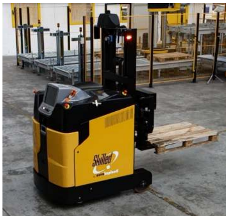
Figure 5: The skilled 1000 autonomous forklift at the Euroimpianti testing facility in Schio.
