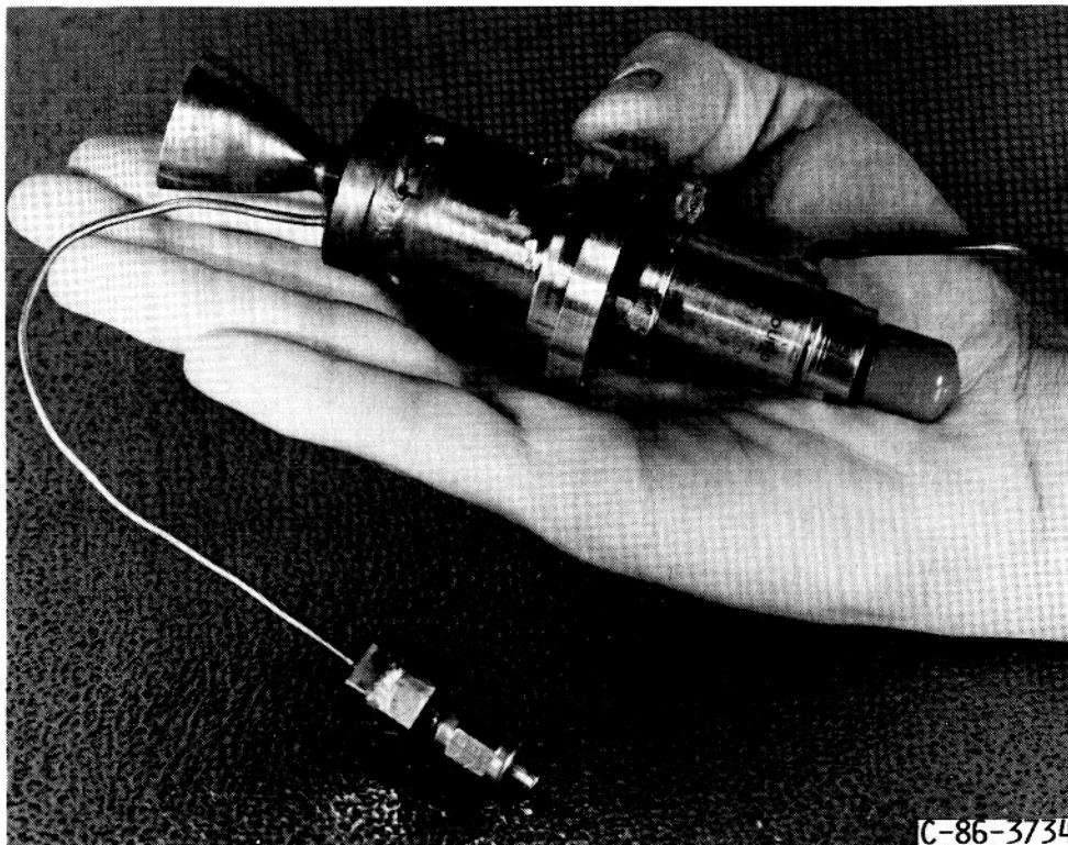
FIGURE 5. - SMALL HYDRAZINE THRUSTER FOR LIFE TESTS.
