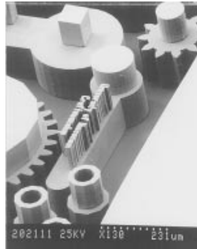
Fig. 10. Double nickel layers of 150 \mu\text{m} height each.
