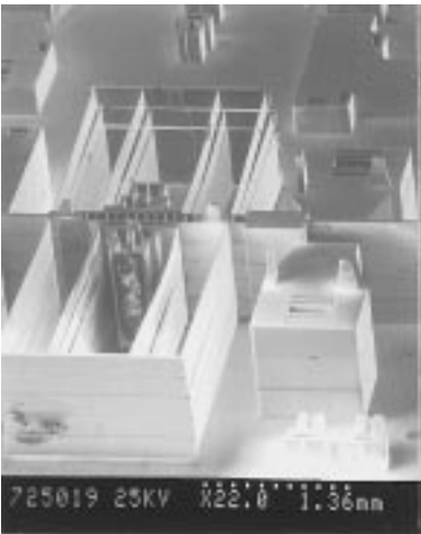
Fig. 15. Linear actuator with 1-mm structural height.
