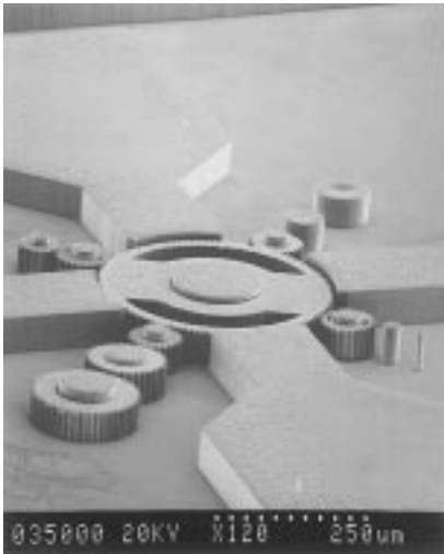
Fig. 3. Assembled nickel structures for friction and magnetic properties testing.
