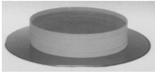
Fig. 8. PMMA bonded to 3-in silicon wafer. The total PMMA height is 1.6 cm.
