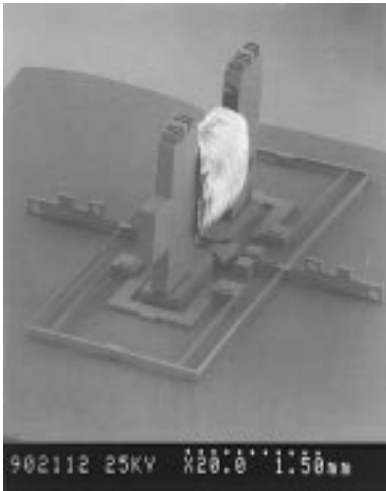
Fig. 14. Linear magnetic actuator with assembled coil. The material is 78-22 permalloy, a soft, very-high-permeability magnetic material that is also used for the coil mandrel.
