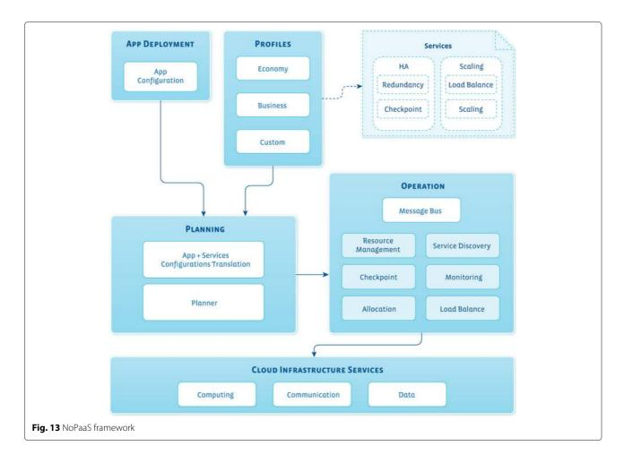
For the developers, it is mandatory to provide a configuration file specifying all information needed to deploy their applications in NoPaaS. Such a configuration file is very similar to what is usually provided to traditional PaaS in order to deploy a new application (e.g., git repository address and multi-tier architecture).
