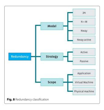
parallel. When one node fails, tasks executing at the failed node can be resumed in any remaining node. In passive redundancy, there is one working replica whereas remaining replicas are standby. When the main node fails, any standby replica can resume failed node tasks. Please note that this active strategy helps to provide load balancing to applications. However, maintaining consistency in the passive model is simpler, and so this strategy is used in different proposals [15].
