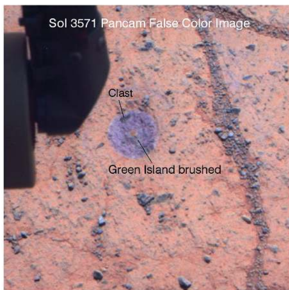
FIGURE 9. Pancam false color image of Green Island, a brushed in situ target. The brushed circle is ~3.8 cm in diameter and is dark as compared to surrounding bedrock because wind-blown dust and sand have been removed. A small rock clast can be seen embedded in the fine-grained matrix of the breccia. The central reddish spot is remnant dust and soil from the brushing activity. Soil-filled fractures are evident on the right side of the image. Generated from Product IDs 1P445203637RADCAG7P2537L2C1, 1P445203721RADCAG7P2537L5C1, and 1P445203794RADCAG7P2537L7C1.
