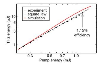
Fig 2. Measured and calculated THz energy versus pump energy at room temperature from cLN.
