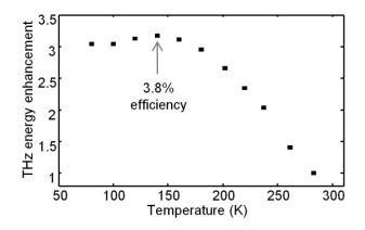
Fig. 4. Efficiency enhancement versus temperature at a fixed pump energy of 1.2 mJ.
