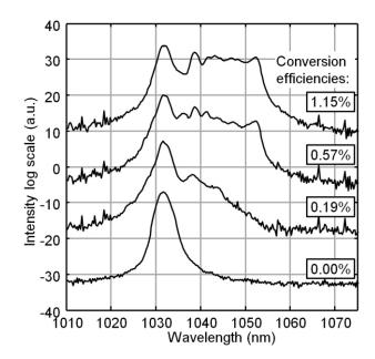
Fig. 3. Spectral broadening of the IR beam after THz generation depending on conversion efficiency.
