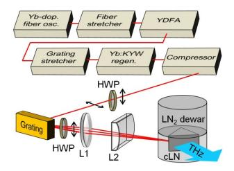
Fig 1. Experimental setup for THz generation. L1: bestform lens with f = 20 cm; L2: Cylindrical lens with f = 15 cm; HWP: Half wave plate at 1030 nm.
