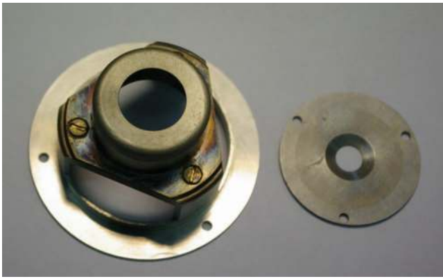
FIG. 2. Puller (22 mm hole) and plasma electrode (10 mm hole).
