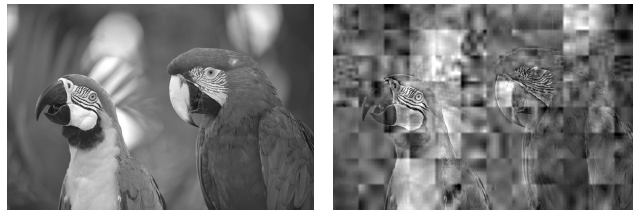
Figure 3. Original encoded image (left, error rate = 10^{-16} , PSNR = 40 dB) and the same image naively stored in unoptimized and untuned approximate cells, with unacceptable quality degradation (right, error rate = 10^{-3} , PSNR = 18 dB).
