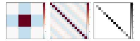
Fig. 2: From left to right: example of a  $3 \times 3$  Laplacian filter, the associated circulant precision matrix  $\mathbf{Q} = \mathbf{\Delta}^{\top} \mathbf{\Delta}$  for convolution with periodic boundary conditions and its counterpart diagonal matrix  $\mathbf{FQF}^{\mathsf{H}}$  in the Fourier domain, where  $\mathbf{F}$  and its Hermitian conjugate  $\mathbf{F}^{\mathsf{H}}$  are unitary matrices associated with the Fourier and inverse Fourier transforms.
