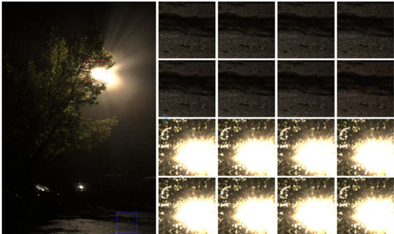
Fig. 13. Visual quality comparison of BigFogMap with different methods at 2.7 bpp. (On the left is the original image, top two rows on the right are non-salient regions of reconstructed image, and two bottom rows on the right are salient ones. From left to right, the first row is original image, official implementation of JPEG XT profile A,B,C, the second row is Choi's method [10], Wei's method [26], Feyiz's method [27], and our proposed method, respectively.)
