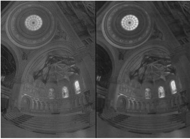
Fig. 12 LCIS rendering (left) and logarithmically compressed rendering. Fine texture details have been preserved for the left rendering. The radiance map was obtained from Ref. 23.
