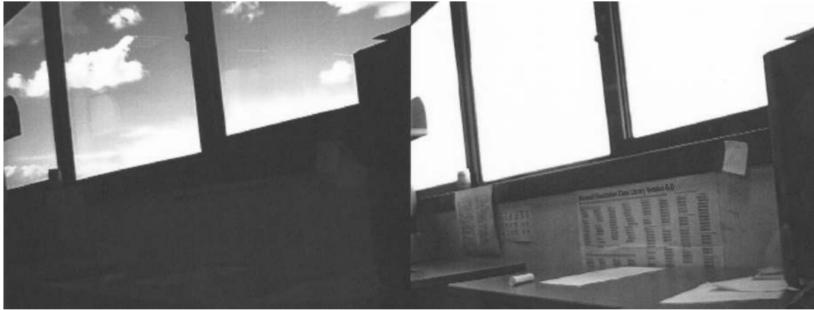
Fig. 7 Two images captured using a CMOS sensor with respectively short and long exposure times. The exposure ratio was not known but roughly estimated to be near 3.5.
