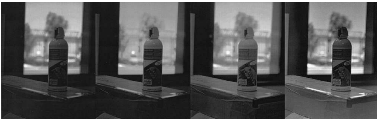
Fig. 9 From left to right, linear gamma corrected, Schlik, histogram adjusted, Retinex compressed rendering for the radiance map recovered (using the parametric model 8,9 ) from the two images of Fig. 5.
