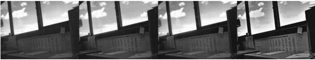
Fig. 10 From left to right, linear gamma corrected, Schlik, histogram adjusted, Retinex compressed rendering for the radiance map recovered (using the parametric model 8,9 ) from the two images of Fig. 7.
