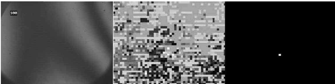
Figure 7 - Detection of a laser spot using the interferogram phase transition algorithm. Left: one frame of the original sequence; middle - processed image; right - processed, binary image showing the position of the target.
