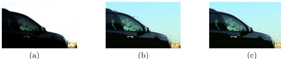
Figure 4. (a) Current frame (long exposure) (b) HDR output without MV refinement in saturated regions (c) HDR output after MV refinement
