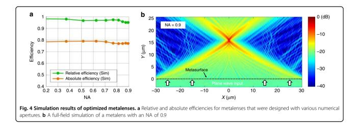
exceed 75%, with approximately 10% of the light reflected from the metalens and 10% absorbed by the silicon. Reflection losses can be reduced via the use of more intricate three-dimensional silicon nanostructures, while absorption losses can be minimized by designing siliconbased devices for longer wavelength operation<sup>28</sup>. A simulated field profile of a metalens with an NA of 0.9 is shown in Fig. 4b, which demonstrates that the lens focuses strongly with minimal spurious diffraction.
