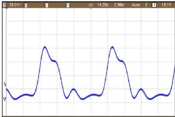
Fig. 7. Drain voltage of the implemented class E amplifier when it operates at 120MHz
