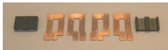
Figure 11. Disassembled current balancing transformer T3.
