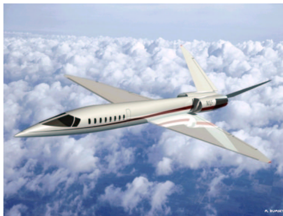
Fig. 2 Natural laminar flow supersonic business jet configuration.
