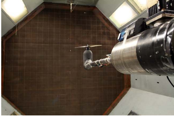
Figure 4. Isolated propeller test configuration in NASA LaRC 12-Foot wind tunnel.
