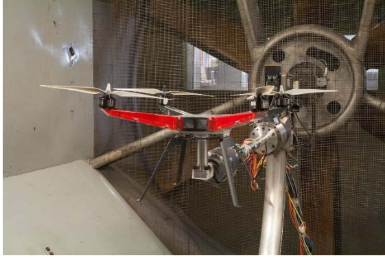
Figure 1. Front view of aircraft model in NASA LaRC 12-Foot wind tunnel.
