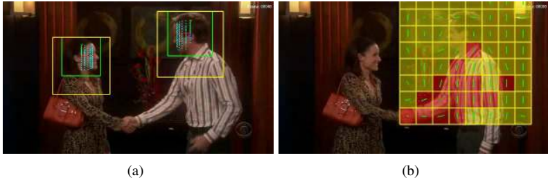
Figure 2: (a) Upper body detections and estimated discrete head orientation. (b) Grid showing dominant cell gradient and significant motion (red cells) for a hand shake.
