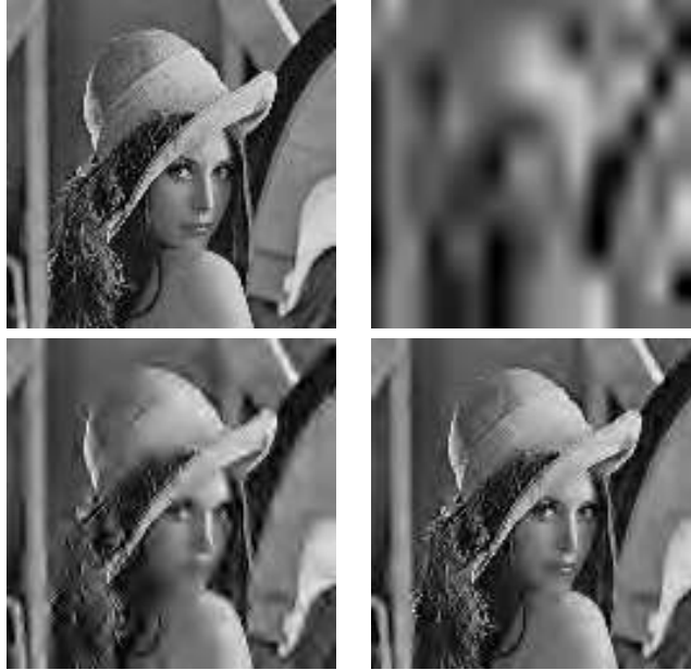
Figure 4. lena image of size 128 \times 128 encoded with JPEG-2000 at 1.7 bpp (top left), and truncated at 0.1bpp (top right), 0.4 bpp (bottom left), and 0.8 bpp (bottom right).
