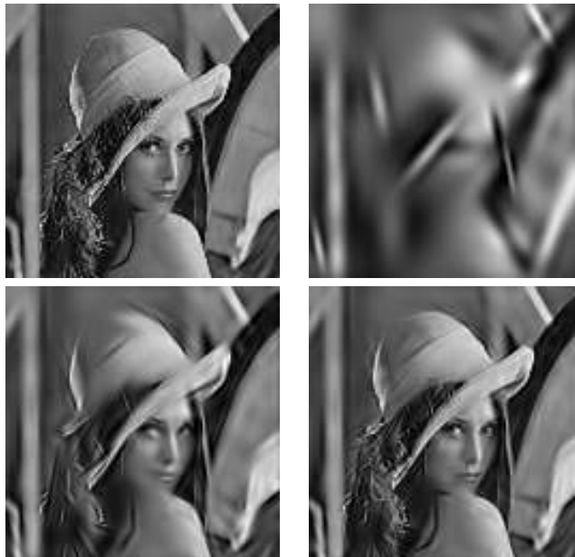
Figure 3. lena image of size 128 \times 128 encoded with MP at 1.7bpp (top left), and truncated at 0.1bpp (top right), 0.4bpp (bottom left), and 0.8bpp (bottom right).
