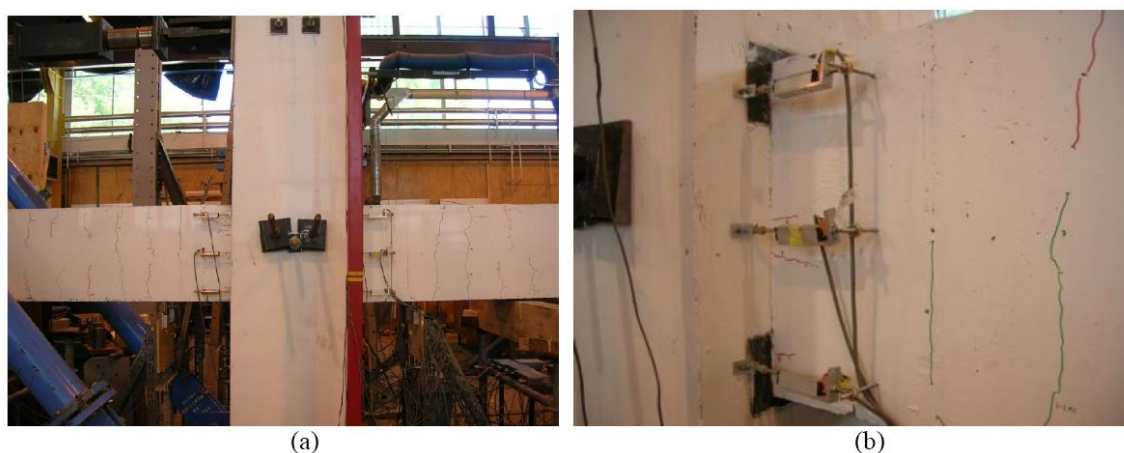
Figure XX: Photographs of the specimen after uni-directional Quasi-Static testing: (a) the specimen at approximately 3 percent drift; (b) the west beam after completion of testing.
