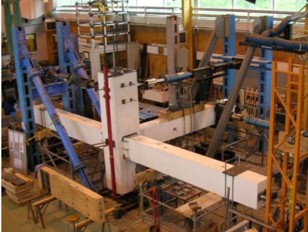
a) Prototype structure showing the location of subassembly (Solberg, 2007); b) Photograph of the subassembly in experimental test apparatus
