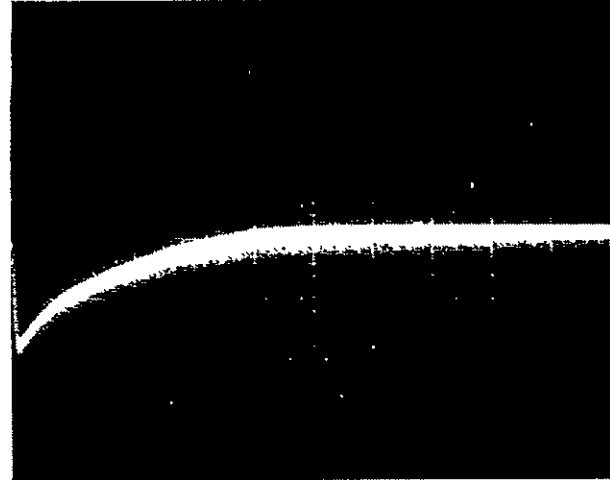
h) LINE — 10V/DIV, 0.5 ms/DIV, Po = 100W, Vin = 130Vdc→110Vdc
