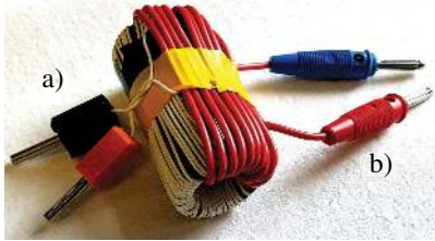
Fig. 6. Stator core equipped with a) Search coil; b) Excitation coil. Remark: Only used for characterization of B-H relationship.
