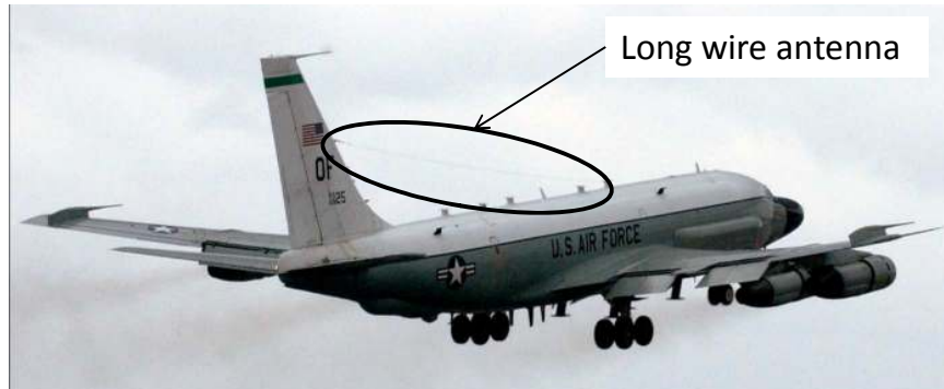
Figure 1.1: Variants of the RC-135 are currently used to detect and analyze signals throughout the EM spectrum. The long wire antenna is used to detect HF signals. (U.S. Air Force photo/Tech. Sgt. Deborah Davis)
