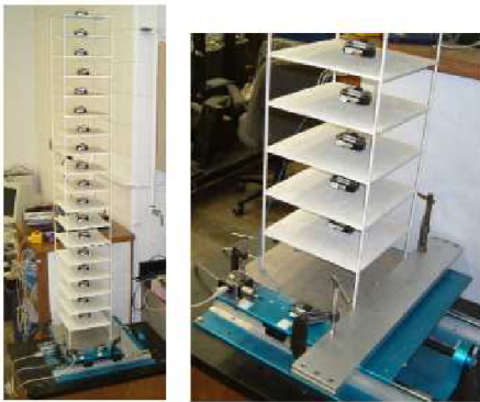
Figure 2: Experimental setup: sensors are attached to an 18-story building model on a shaking table.
