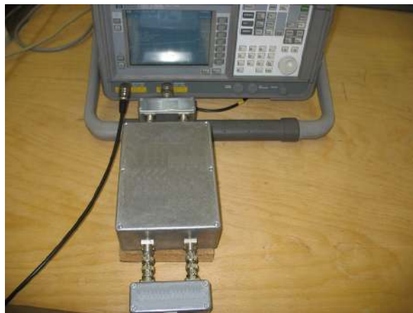
Fig. 14. EMI filter characterization
