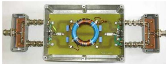
Fig. 15. Experimental EMI filter characterization for CM
