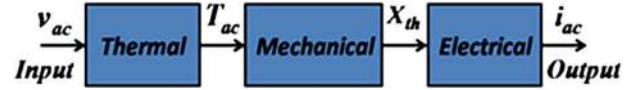
Fig. 2. (a) Block-diagram demonstration of the thermoelectromechanical model of the resonator that can be divided into three subsystems of thermal, mechanical, and electrical nature. The electrical input ac voltage causes a temperature fluctuation that is turned into an ac mechanical force and, therefore, displacement. Finally, the mechanical displacement is turned into an electrical signal (motional current) due to the piezoresistive effect.
