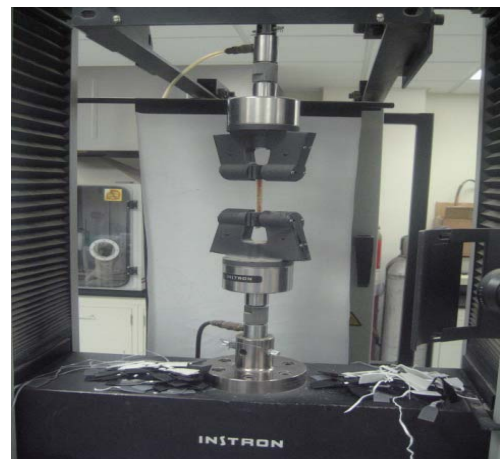
Fig. 9 Clay/polymer nanocomposite sample during mechanical test.
