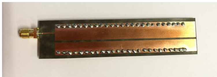
Figure 13. Fabricated Antenna Structure
