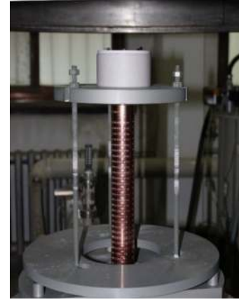
FIG. 1. Main cell stack for diffusion bonding in Tsinghua University.
