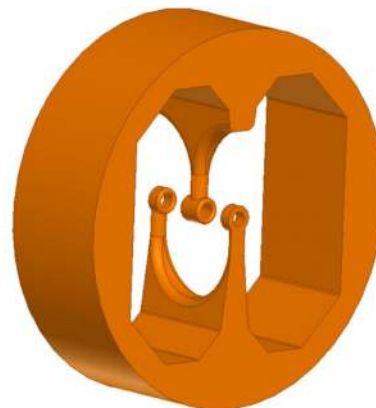
FIG. 9. Regular cell design (left) and assembly view (right) of the IH 750 MHz cavity.
