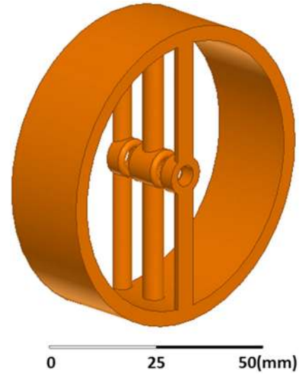
FIG. 11. The 5 MeV reference 3 GHz DTL cavity.
