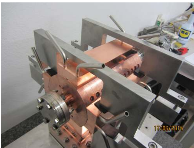
FIG. 13. The 3 GHz BTW prototype.
