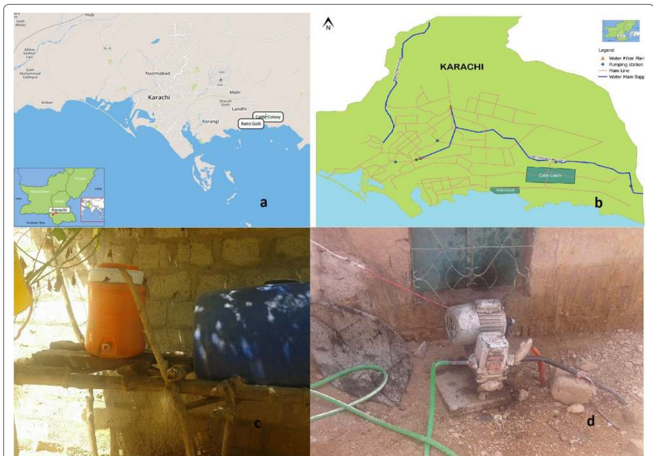
Fig. 1 Study areas in Karachi and water supply and consumption; a Map of Cattle Colony and Rehri Goth in the Bin Qasim Town of Karachi (Insets show location of Karachi within Pakistan and Pakistan in South Asia); b water distribution system in Karachi showing piped water supply to study areas from a natural lake east of Karachi; c water storage tanks used in some households; and d pressure booster pumps used by consumers to overcome low pressure and intermittent supply of piped water
