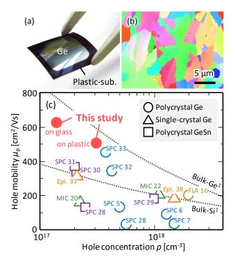
**FIG. 4.** (a) Photograph and (b) EBSD image of the SPC-Ge layer formed on a GeO<sub>2</sub>-coated plastic substrate where t = 400 nm and  $T_g = 375$  °C. (c) Comparison of the hole mobility  $\mu_p$  and hole concentration p of Ge(Sn) films on insulators. The growth method and the reference number are shown near each symbol. The data for single-crystal bulk Si and Ge are shown by dotted lines [Ref. 1].
