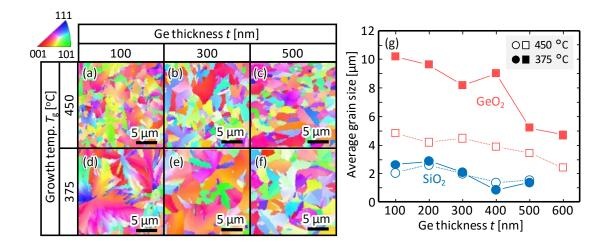
**FIG. 2.** Grain size of the SPC-Ge layers on a GeO<sub>2</sub>-coated glass substrate. (a)–(f) EBSD images as a matrix of *t* and  $T_g$ . The colors indicate the crystal orientation, according to the inserted color key. (g) Average grain size determined by the EBSD analyses with  $T_g = 450 \text{ °C}$  and 375 °C as a function of *t*. The data for the sample without GeO<sub>2</sub> (named SiO<sub>2</sub> sample) are shown for comparison.
