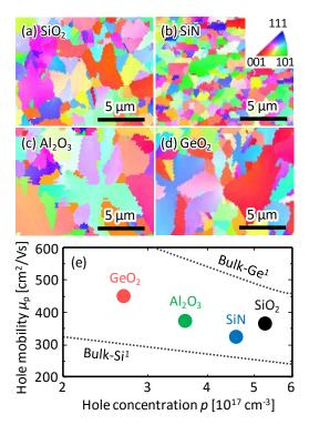
FIG. 1. Characteristics of the SPC-Ge layers for t = 300 nm and  $T_g = 450$  °C, grown on various underlayers (SiO<sub>2</sub>, SiN, Al<sub>2</sub>O<sub>3</sub>, and GeO<sub>2</sub>) formed on a glass substrate. (a)–(d) EBSD images of the Ge layers, where the colors indicate the crystal orientation, according to the inserted color key. (e) Comparison of hole mobility  $\mu_p$  and hole concentration p of the samples. The data for single-crystal bulk Si and Ge are shown by dotted lines [Ref. 1].
