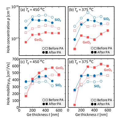
**FIG. 3.** Electrical properties of the SPC-Ge layers before and after PA (500 °C) as a function of *t*. (a),(b) Hole concentration *p* and (c),(d) hole mobility  $\mu_p$  for the GeO<sub>2</sub> and SiO<sub>2</sub> samples where  $T_g = (a),(c) 450$  °C and (b),(d) 375 °C. The data before PA are shown by open symbols and after PA by closed symbols.
