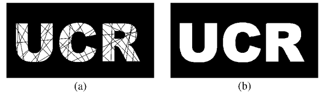
Fig. 9. Dilation example. (a) Crisscrossed UCR logo; (b) clean UCR logo following dilation.
