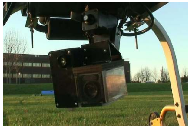
Figure 2. On-board camera system mounted on a pan-tilt unit.
