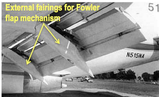
(a) An example of external fairings for Fowler flap mechanism. 6
