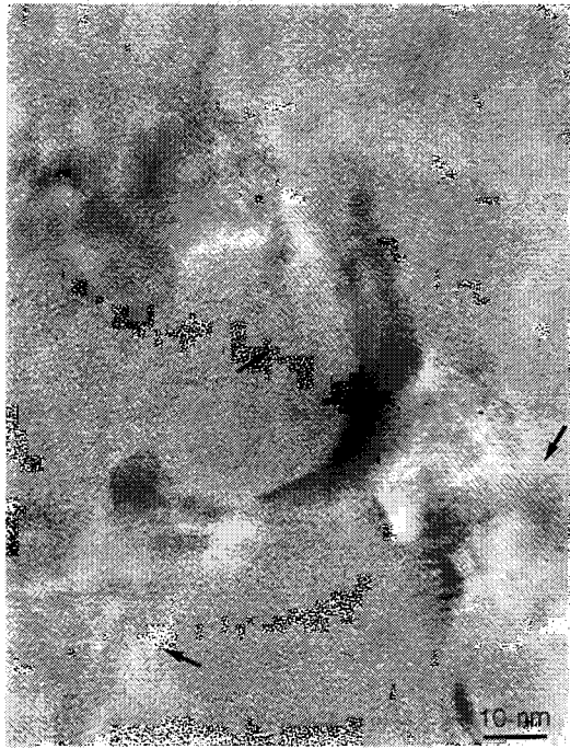
Fig. 6 High-resolution electron micrograph of a rapidly solidified \text{Al}_{92}\text{Mn}_6\text{Ce}_2 alloy.
