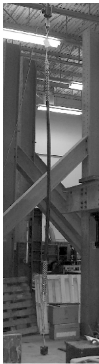
Fig. 16. Mesh Grip Strength Test Setup
