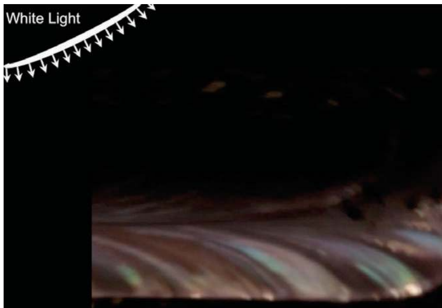
Movie 3. Structural color observed for printed eutectic filaments. Top view of printed eutectic filament (2 mm wide, v = 0.35 \text{ mm}\cdot\text{s}^{-1} ) reveals that their structural color (blue) switches on and off depending on orientation of lamellar features with respect to the white light source.
