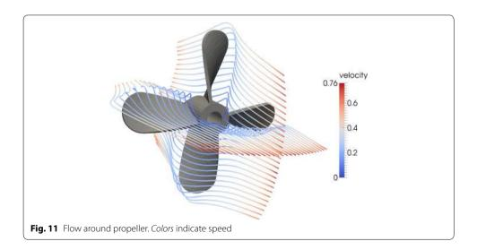
continuity of the streamlines of the velocity going from the finite element space defined on the background mesh to the finite element space defined on the overlapping mesh surrounding the propeller.
