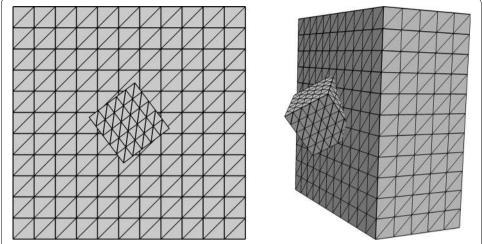
**Fig. 6** Location of the overlapping domain in the background mesh. The domain  $\Omega_1$  is placed in the center of  $\Omega$  and rotated along the z-axis in 2D (*left*) and along the y- and z-axes in 3D (*right*)
