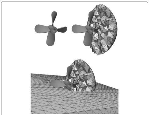
**Fig. 10** Propeller geometry and meshes. Propeller geometry (*top left*) and body-fitted mesh (*top right*). Non body-fitted background mesh and propeller (*bottom*)
