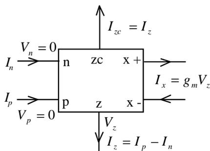
Fig. 1: Active CDTA element containing the “zc” terminal, which provides a copy of the current  $I_z$ .
