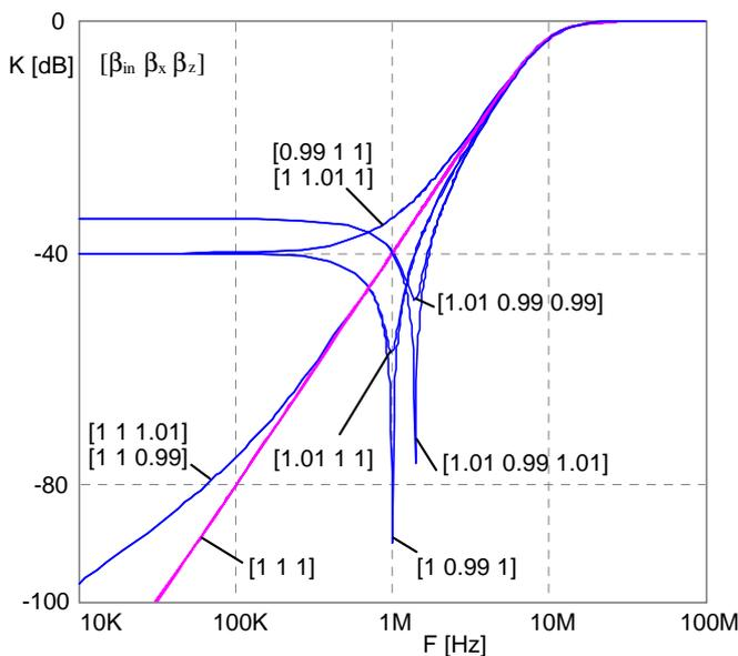
Fig. 3: The HP responses affected by different tracking errors. PSpice analysis with ideal model of the CDTA.
