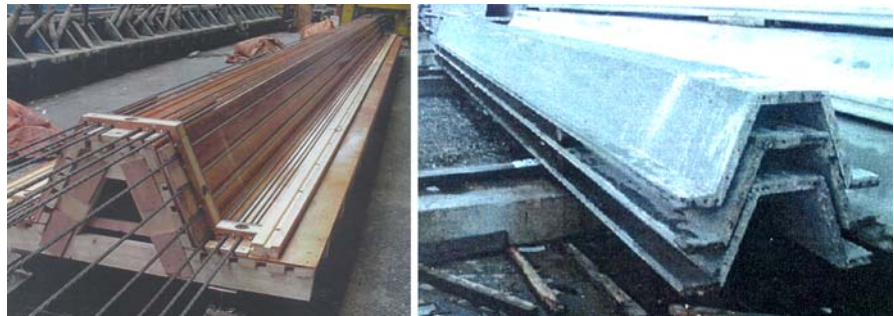
Fig. 4 HPFRC sheet piles prestressed with strands 3/8"
