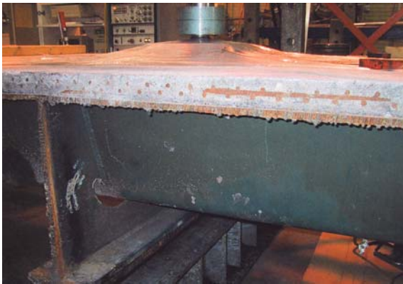
Fig. 2 Fatigue test on a steel girder provided with an overlayer of HPFRC [4]
