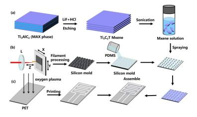
**Figure 1.** (a) Preparation of  $Ti_3C_2T_x$  MXene. (b) Preparation of Micro-Patterned MXene/PDMS conductive film. (c) Assembly of the MXene-based piezoresistive sensor.
