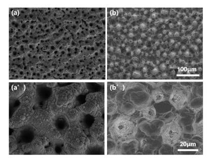
**Figure 2.** (**a**,**a**') The top-view SEM images of the filament-processed silicon mold surface under low and high magnifications. (**b**,**b**') Differently magnified SEM images of the fabricated MXene-based PDMS film surface.
