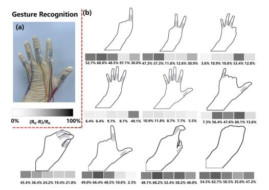
**Figure 7.** (a) The gesture recognition glove based on the fabricated piezoresistive sensor. The prepared five MXene-based piezoresistive sensing devices were assembled at the joints of the glove fingers. (b) Gestures of Arabic numerals and their corresponding responsive output.
