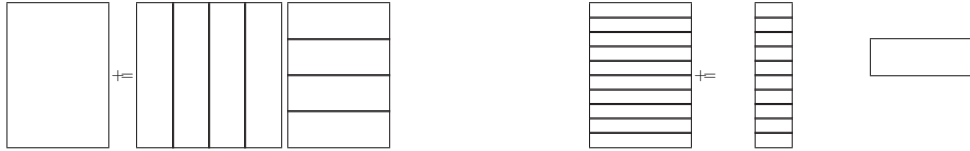
Figure 2: Left: Partitioning of A and B . Right: Blocking for one individual panel-panel multiplication (GEPP) operation, C := A_j B_j + C .
