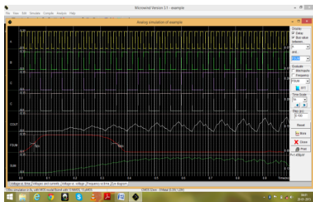
Figure 6:Simulation Results for SR-Latch using CD Logic.
