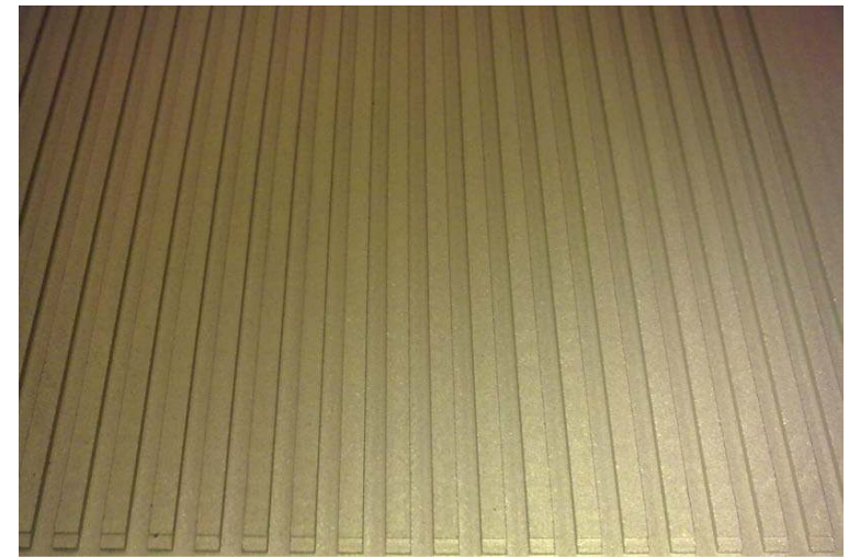
Bipolar plate channels, nitrided plate
