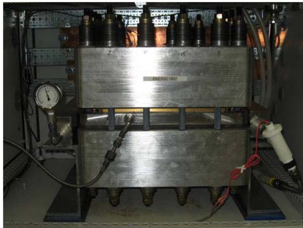
0.6 ft 2 cell stack, >10,000 cell hours, ~1 kg/day/cell
