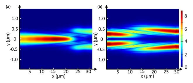
Figure 5: Simulated light propagation in the designed power splitter for the launched  $TE_0$  (a) and  $TE_1$  (b) modes.
