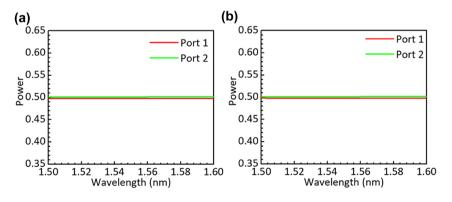
Figure 6: Simulated power splitting ratio of the designed power splitter for the  $TE_0$  (a) and  $TE_1$  (b) modes.
