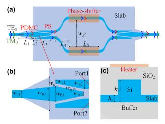
**Figure 1:** Schematic configuration of the proposed polarization switch. (a) The top view; (b) the PDMC and PS regions; and (c) the cross-section of the ridge waveguide of the phase shifter.
