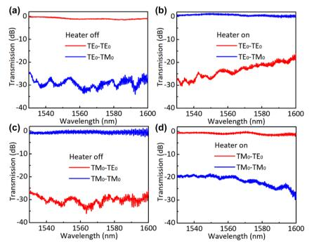
**Figure 10:** Measured transmissions of the fabricated polarization switch for the launched  $TE_0$  (a) and  $TM_0$  (b) modes when it is off; measured transmissions of the fabricated polarization switch for the launched  $TE_0$  (c) and  $TM_0$  (d) modes when it is on.
