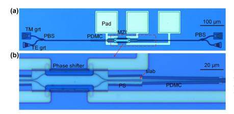
**Figure 9:** The optical microscopy images of the fabricated polarization switch. (a) The optical microscopy images for the fabricated polarization switch with two PBSs; and (b) the enlarged view of MZI with power splitters and phase shifters.
