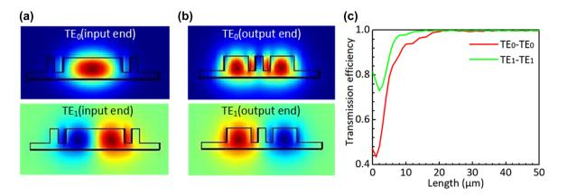
**Figure 4:** The mode profiles of the TE<sub>0</sub> and TE<sub>1</sub> modes at the input end (a) and the output end (b) of the triple-core waveguide of the PS. (c) Simulated conversion efficiencies of the TE<sub>0</sub>–TE<sub>0</sub> and TE<sub>1</sub>–TE<sub>1</sub> in the triple-core waveguide as the length  $L_3$  varies.
