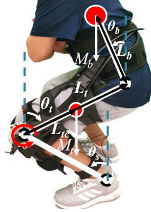
Fig. 9 Quasi-static model used to derive the assistive knee joint torque during squat motion.
