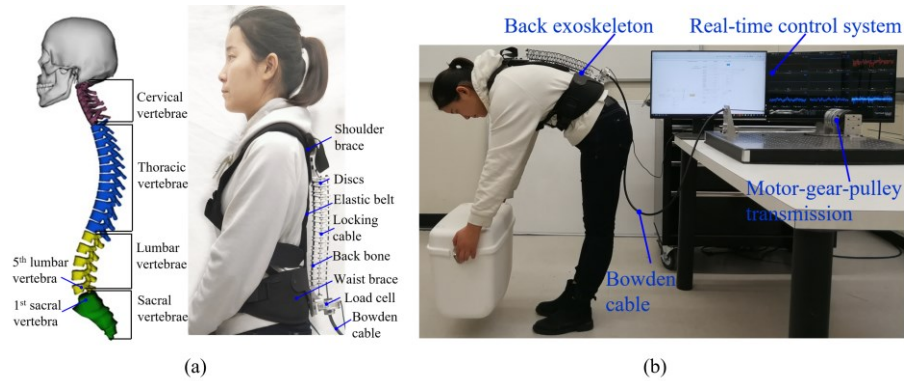
600 Fig. 15 (a) The spine-inspired back exoskeleton leverages on a hyper-redundant continuum mechanism. Thanks to its compliance, this wearable robot provides assistive force while being conformal to the anatomy of the human back and unobtrusive for natural motion. (b) A healthy subject wearing the back exoskeleton to perform stoop lifting of a 15 kg load. The spine continuum mechanism is powered by a tethered actuation platform via Bowden cable 605 transmission.
